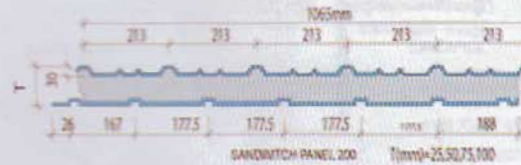
SANDWICH PANEL 200 f(\text{mm})=25,50,75,100
